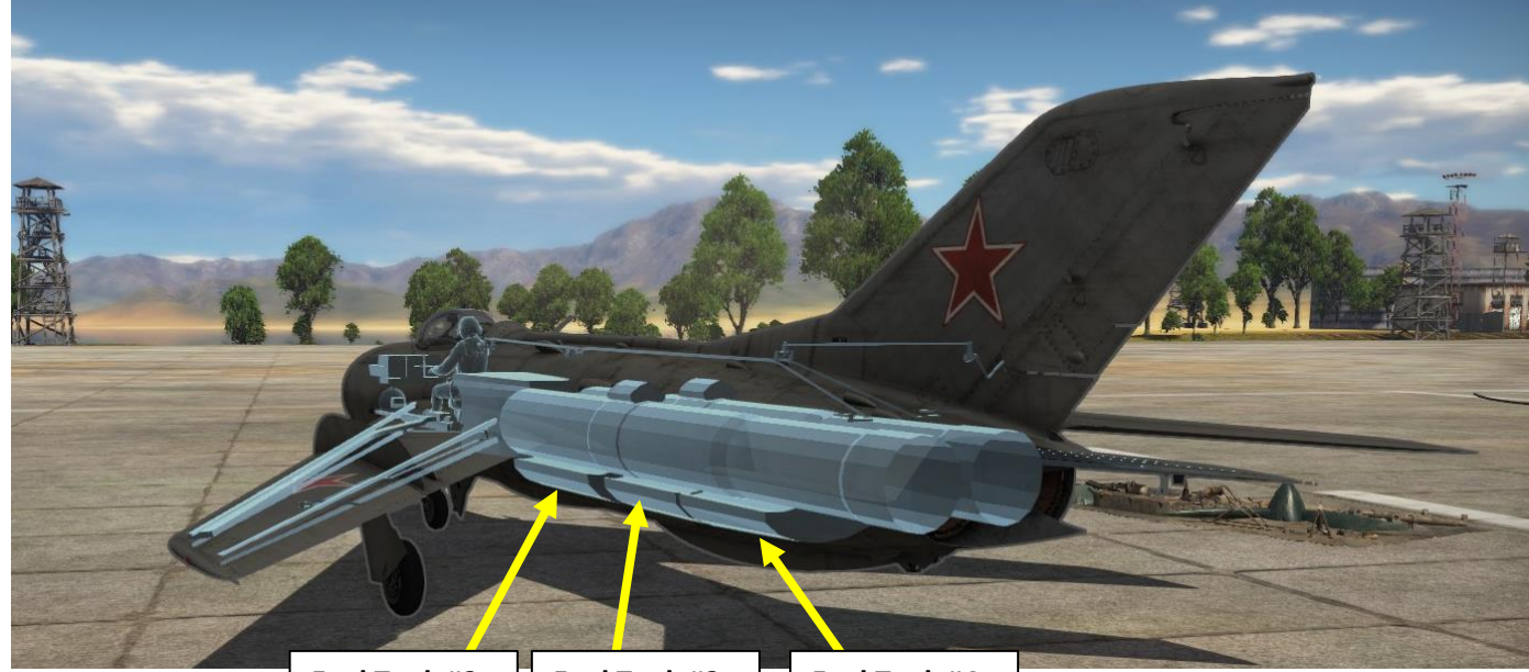
Fuel Tank #2 (330 liters) Fuel Tank #3 (180 liters) Fuel Tank #4 (175 liters)
