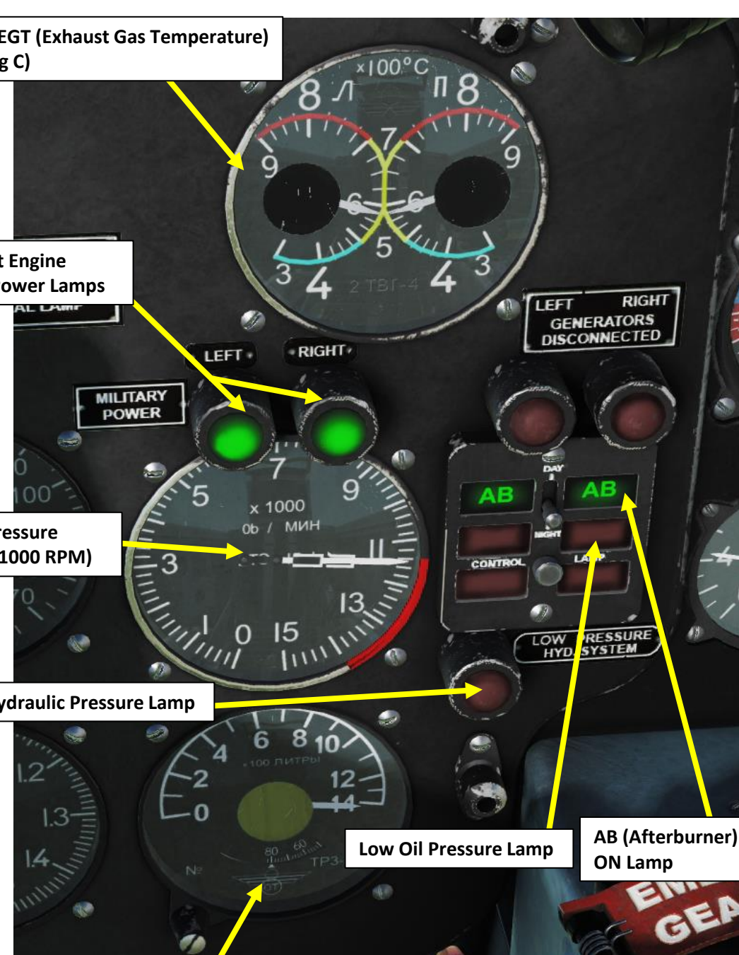
Fuel Flow Meter (x100 Liters/hour)
