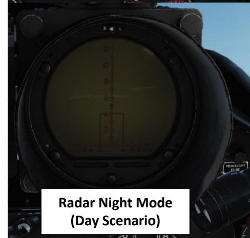
RP-5 Izumrud Radar Mode Selector • Mode 1: Use below 2000 m (Low Altitude Mode) • Mode 2: Use above 2000 m
