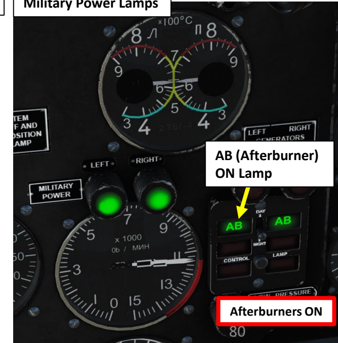
Left/Right Engine Military Power Lamps
