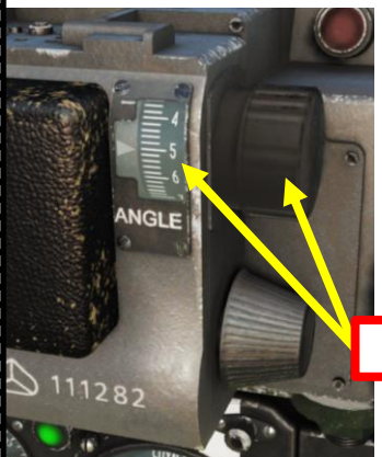
Throttle Twist Grip (ASP-5N Gunsight Distance to Target Selector in hundreds of meters)
